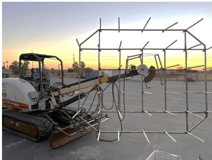
Figure 3. Newly designed canopy shaker built for mature, large olive trees in California.
