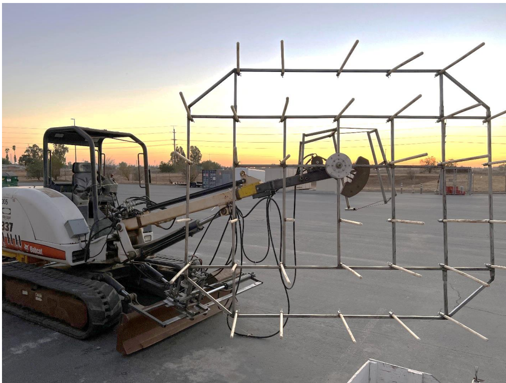
Figure 2. Newly designed canopy shaker built for old large olive trees in California.
