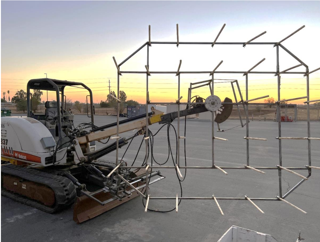
Figure.4 Newly designed canopy shaker built for old large olive trees in California.
