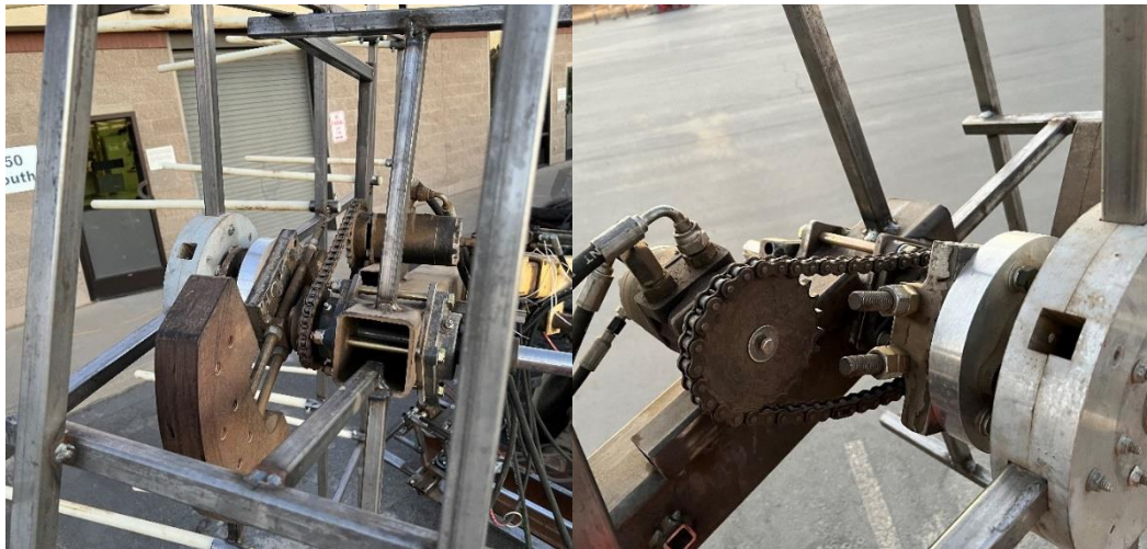
Figure.5 Internal mechanism used to generate circular oscillation movement in the canopy shaker.
