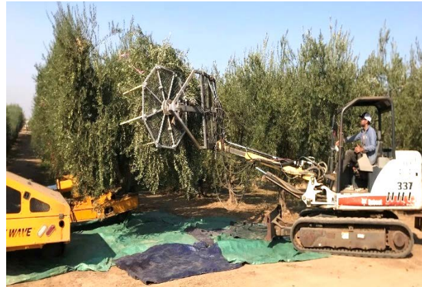
Figure 5 Trunk shaker and canopy shaker, shaking an olive tree simultaneously
