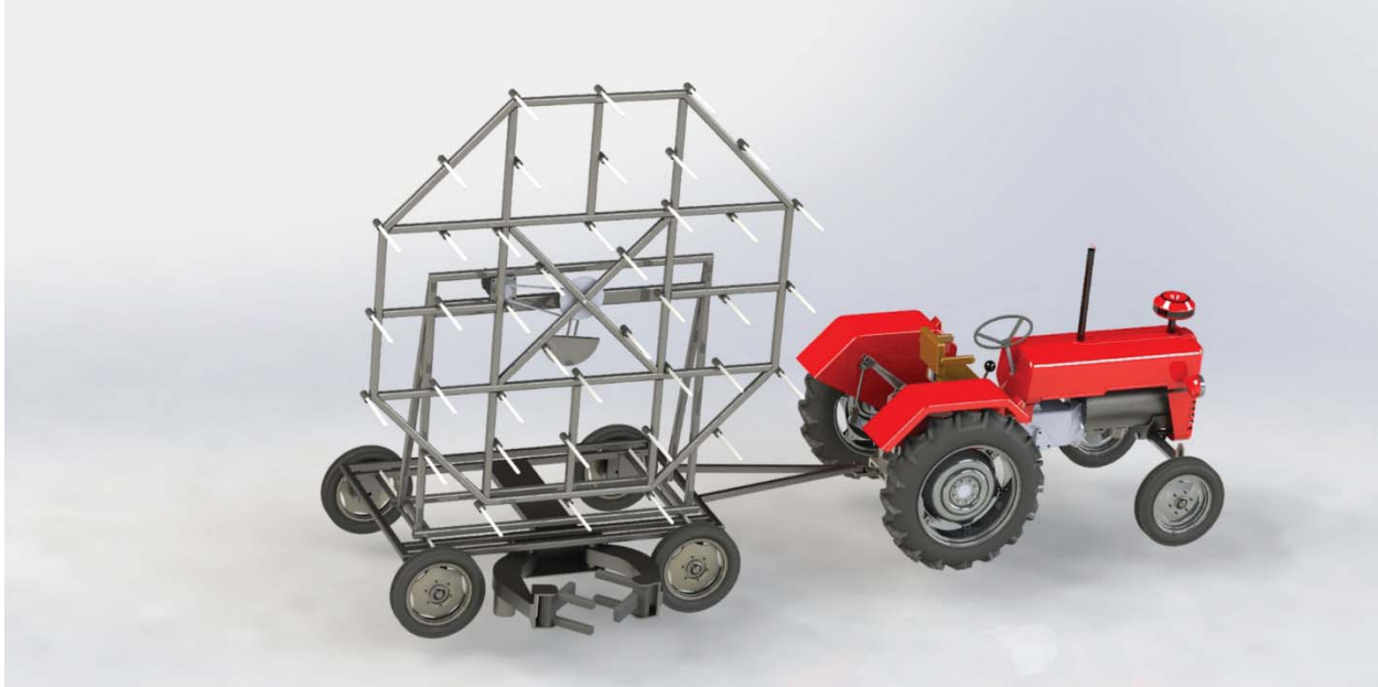
Figure 8. Proposed shaker design that includes both canopy shaker and trunk shaker components.
