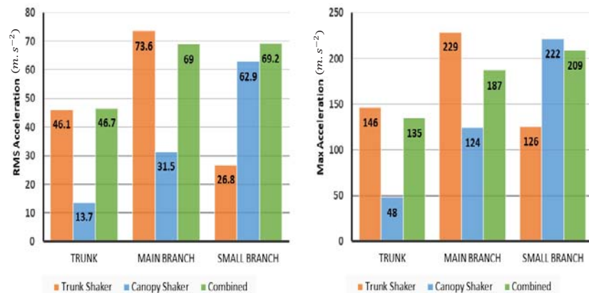
Figure 3. Root mean square of vibration measured at each part of a tree (left) and maximum acceleration produced by the two harvesters at each part of a tree (right).
