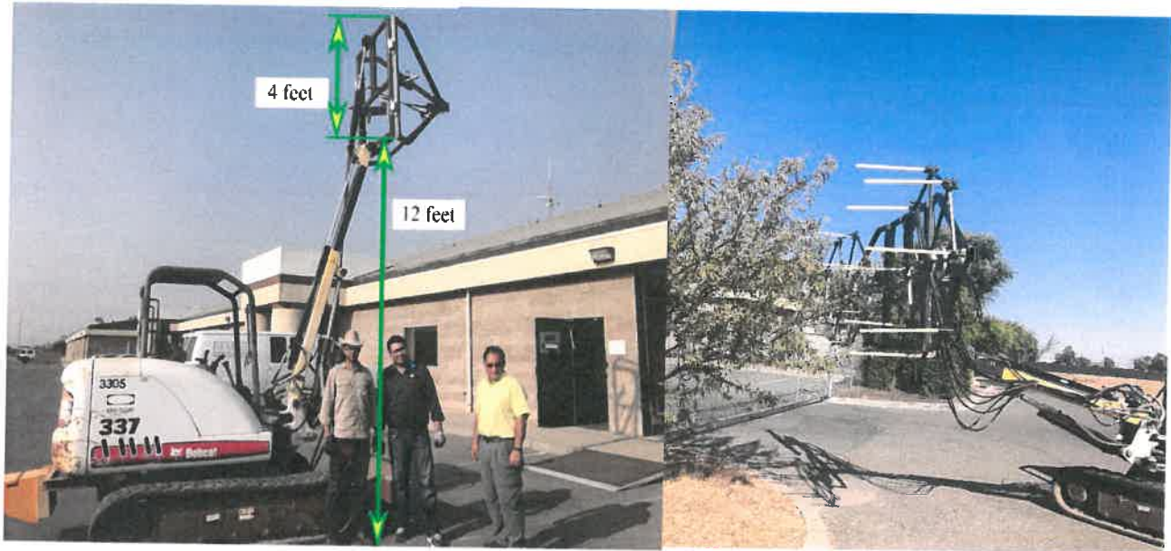
Figure 7. Head frame attached to the Bobcat 337. Harvesting head can rise up to 12 feet from ground and harvest trees up to 16 feet.
