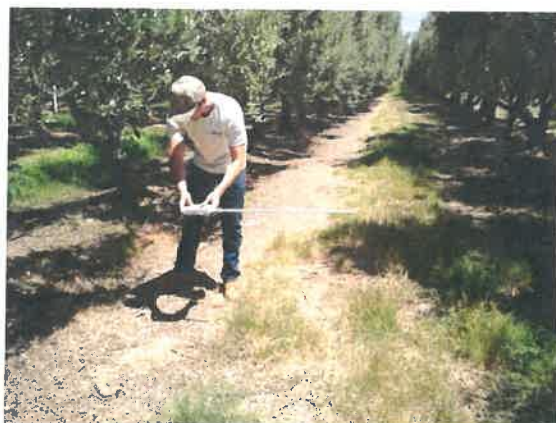
Figure 3. Measuring light levels using a point PAR sensor in the canopy (left) and using a quantum sensor (right) following hedging
